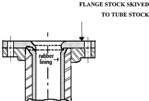
**FIGURE B11.10** Flange face rubber lining.
