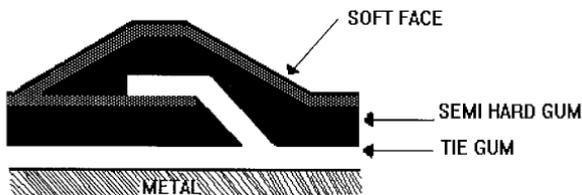
**FIGURE B11.4** Multiple construction lining (3-ply shown).
