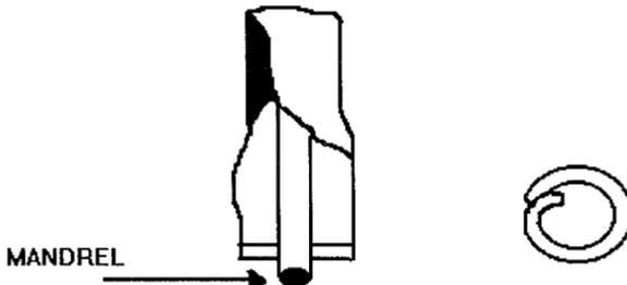
FIGURE B11.5 Method of building tube.
