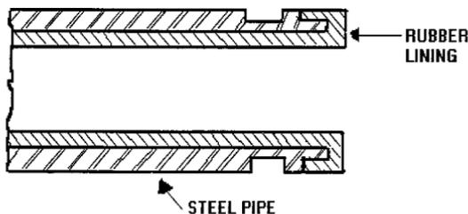
**FIGURE B11.14** Rubber lining of grooved pipe.
