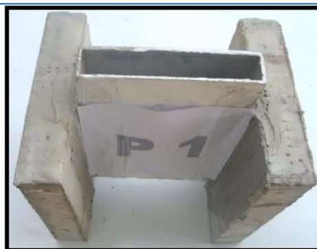
Fig. 3 Push out specimen
