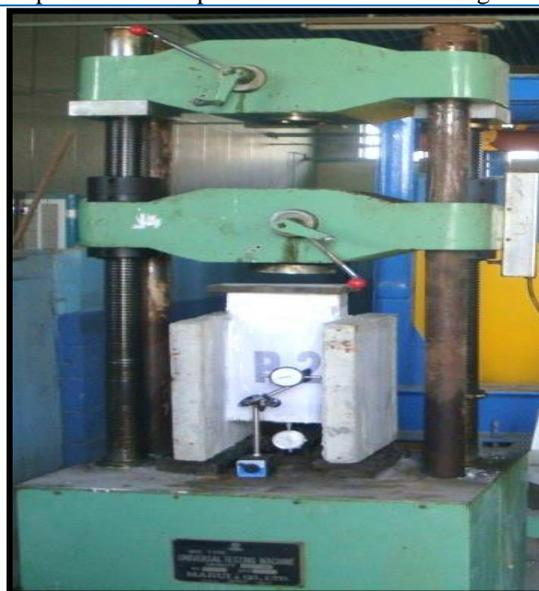
Fig. 4 Push-out test arrangement
