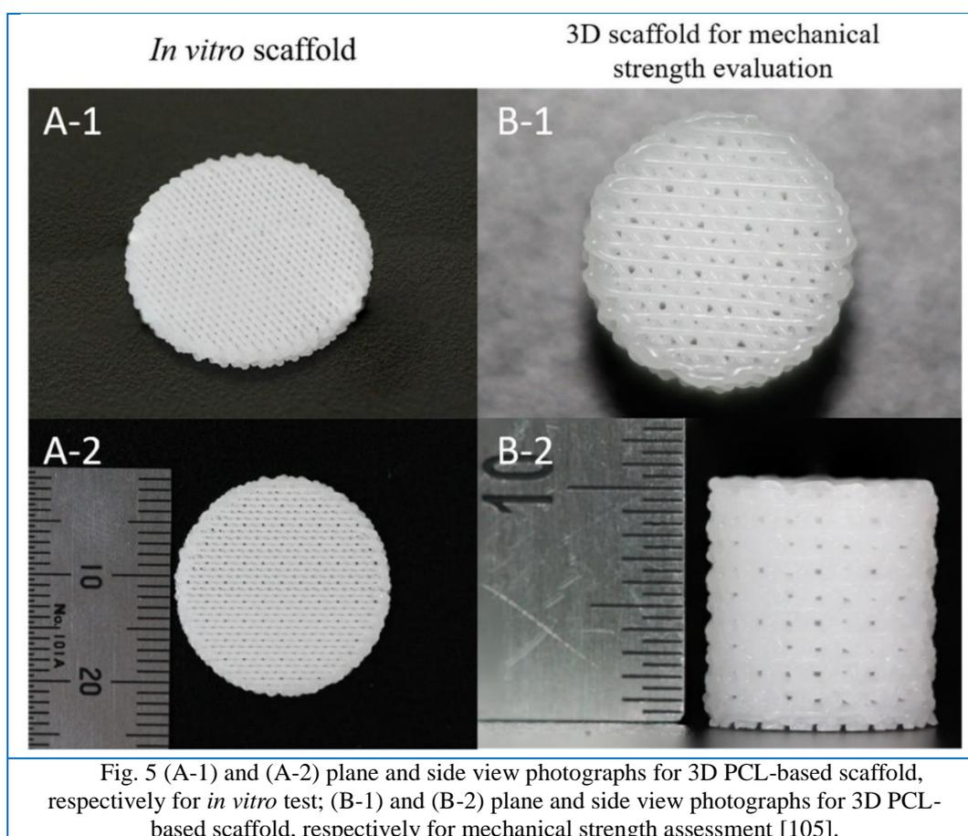
Fig. 5 (A-1) and (A-2) plane and side view photographs for 3D PCL-based scaffold, respectively for *in vitro* test; (B-1) and (B-2) plane and side view photographs for 3D PCL-based scaffold, respectively for mechanical strength assessment [105].
