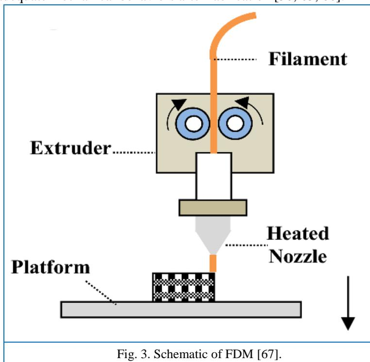
Fig. 3. Schematic of FDM [67].
