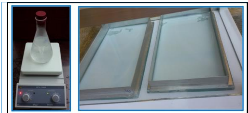
Fig. 3 Preparation of PMMA/SiO 2 composite sheets.
