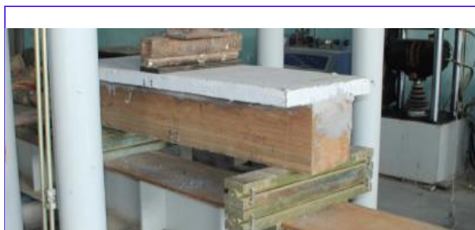
Fig. 11 specimen TF1 before failure
