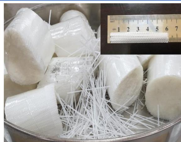
Fig. 3. Polyolefin fiber.
