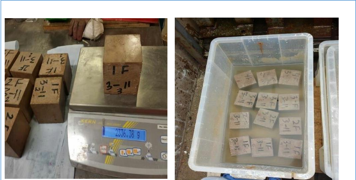
Figure 7: A- Water absorption test
