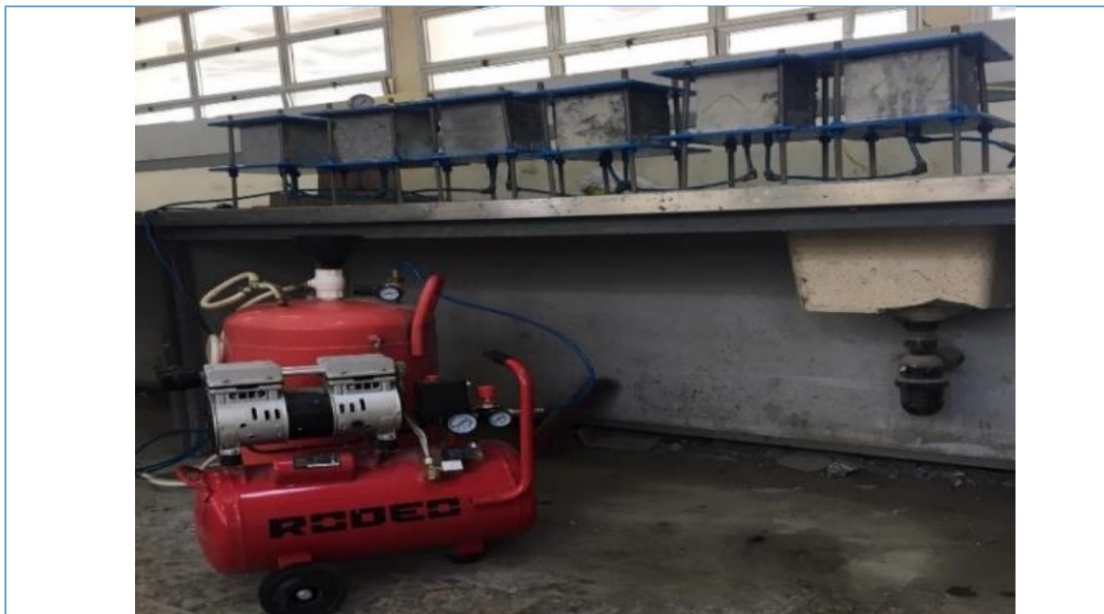
Figure 2: Device of the water penetration test.
