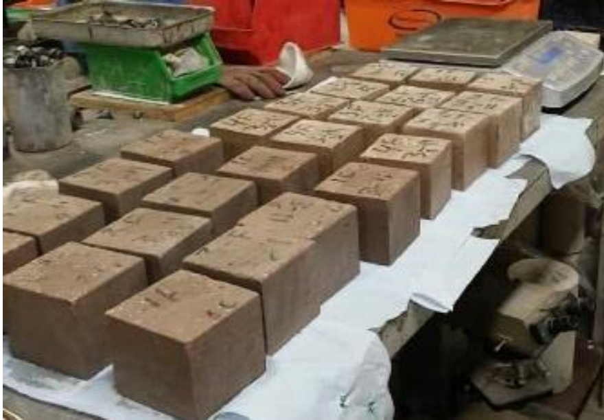
Figure 7: B- Water absorption specimen test
